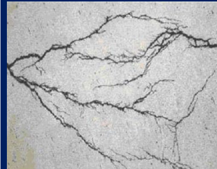
Chloride Stress Corrosion Cracking
