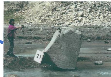
Debris from the entrance building arch, found 370 m away (weight: 15 t).
