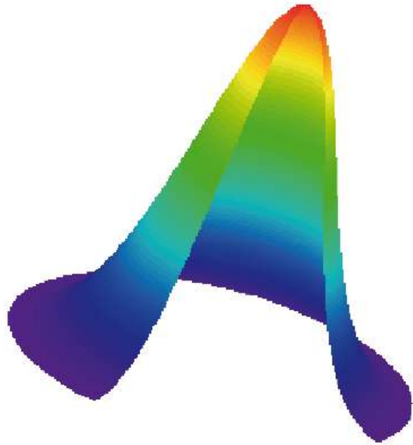
Figure 2a. The three-dimensional field-intensity distributions on the rectenna for the Gaussian beam.
