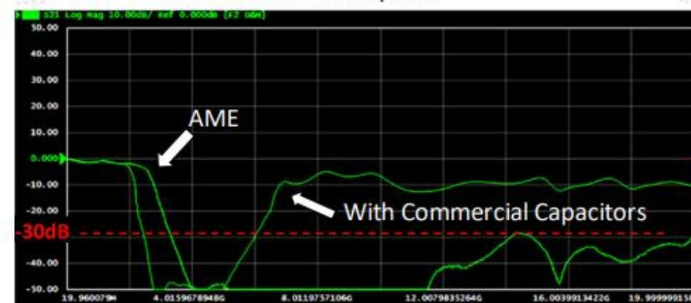
LPF with AME Capacitors filters the signal at least up to 20GHz. (less than -30db)
