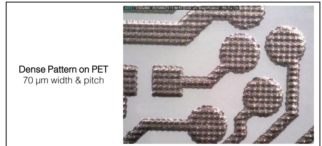
4) Application: very narrow & dense conductive patterns
