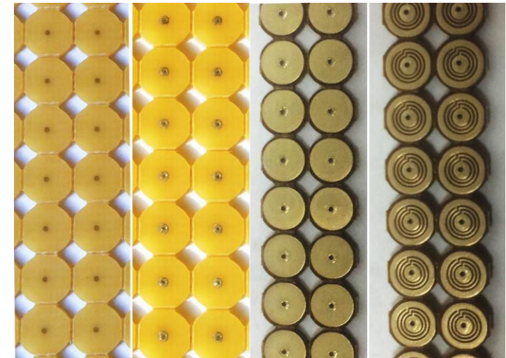
Special Heater on FR4, Inkjet printed 600 \mu\text{m} vias
