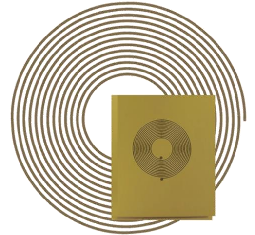
Coil with 18 Turns Linewidth 70 \mu\text{m} . Pitch 70 \mu\text{m} .
