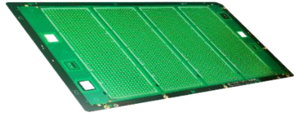
4-Layer PCB Resistivity < 6 \mu\Omega\text{cm} , Thickness 20 \mu\text{m}
