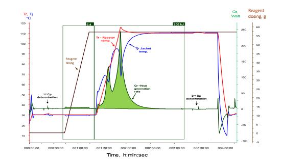
No heat release during the dosing. The heat release starts <u>after</u> the dosing (uncontrolled, dangerous reaction)
