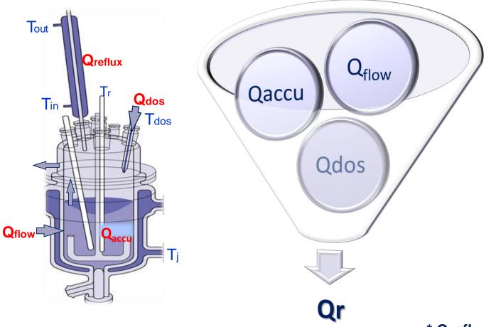
**Q**<sub>flow</sub>- The heat flow across the reactor wall
