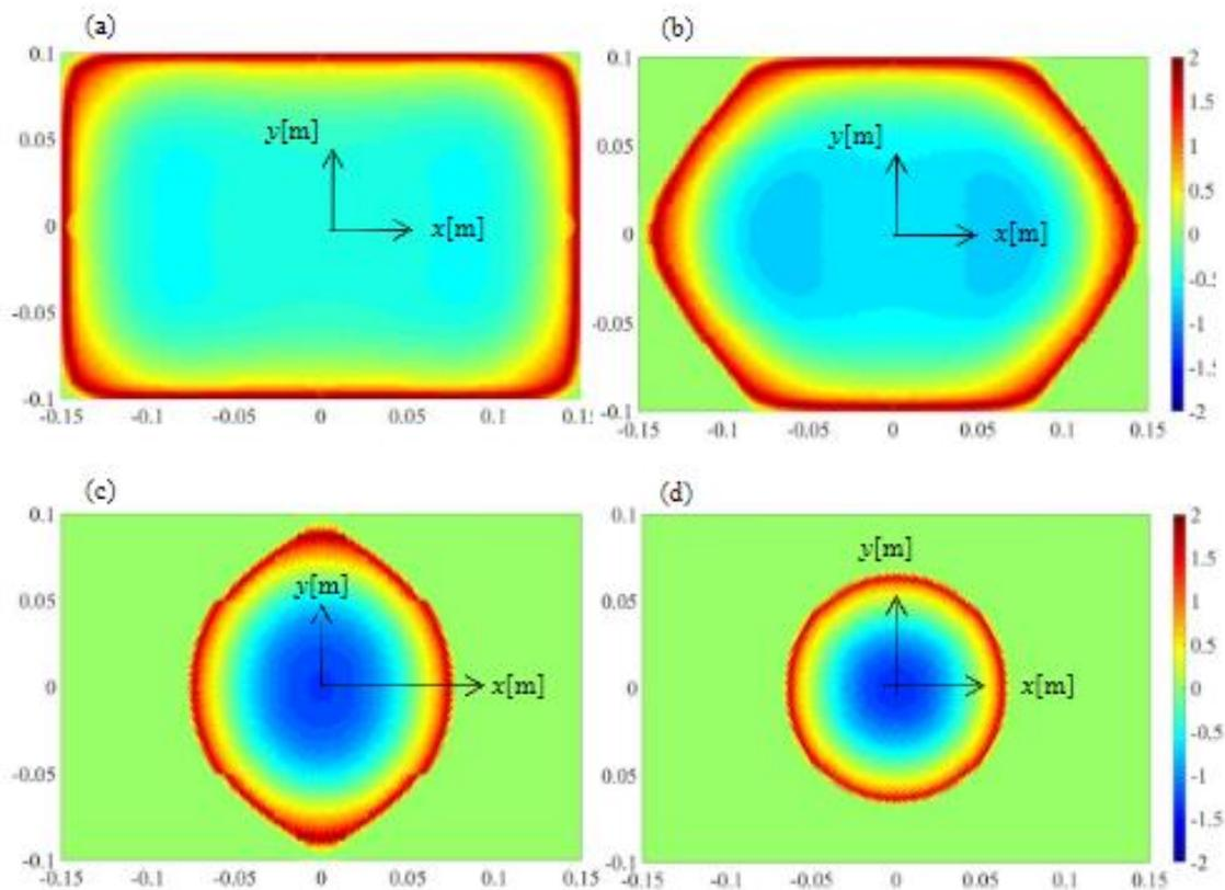
*Figure 1 – Progressive debonding fronts at the substrate adhesive interface of a rectangular tile subjected to uniform heating*
