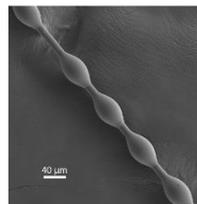
*Figure 1 - Intermittently spaced epoxy beads on fibre*
