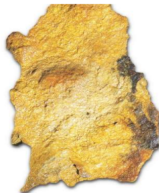
Yellow – Brown \text{FePO}_4 + \text{H}_3\text{PO}_4
