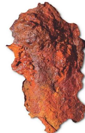
Red – brick - brown \text{Fe}(\text{OH})_3, \text{FeOOH}, \text{Fe}_2\text{O}_3 \cdot n\text{H}_2\text{O} + \text{H}_2\text{O}, \text{O}_2
