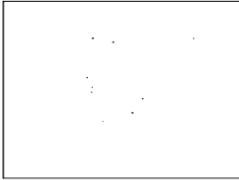
Rust Grade 9-G, 0.03% Rusted
