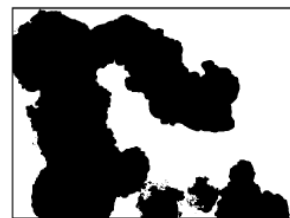
Rust Grade 1-S, 50% Rusted
