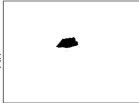
Rust Grade 8-S, 1% Rusted
