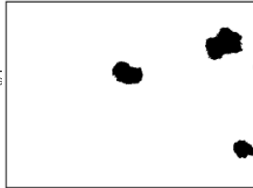
Rust Grade 5-S, 3% Rusted
