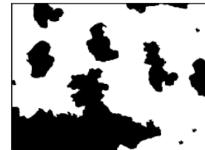
Rust Grade 2-G, 33% Rusted
