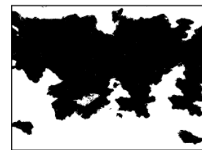
Rust Grade 1-G, 50% Rusted
