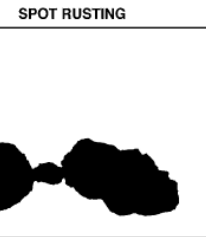
Rust Grade 3-S, 16% Rusted
