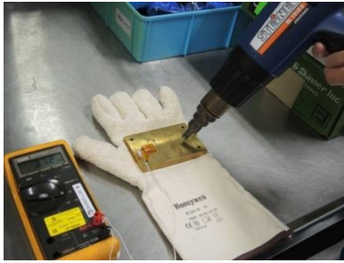
Figure 4: Measuring soldering material's melting point
