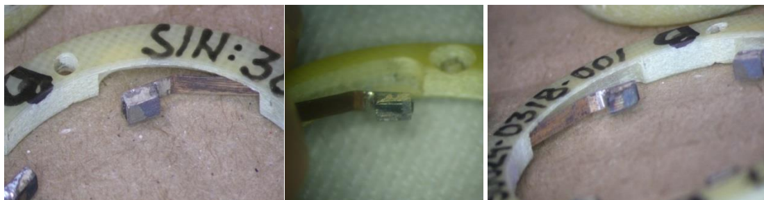
Figure 6: a, b and c (left to right): Results of visual examination of brand-new brushes: Different brush dimensions and uneven contact surface.
