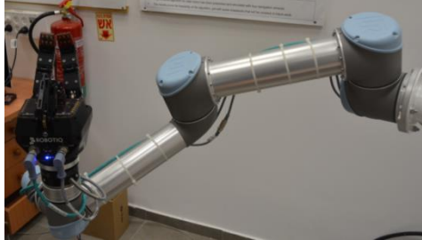
Figure 4 - Takktille sensors on the 3 Finger Gripper
