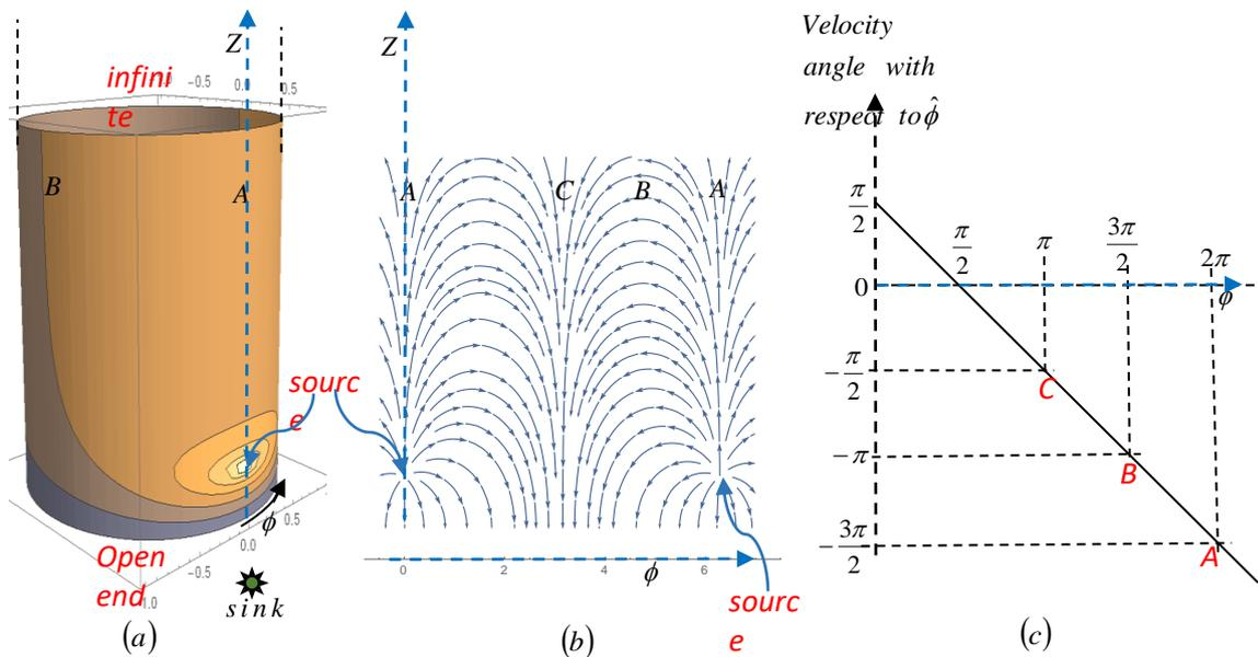
Figure 1: Asymptotic behaviour of the ow on a semi-infinite open cylinder affected by one source: (a) Equi-pressure contours and (b) Streamlines of the field ow; (c) The angle of the velocity vector with respect to  $\hat{\phi}$
