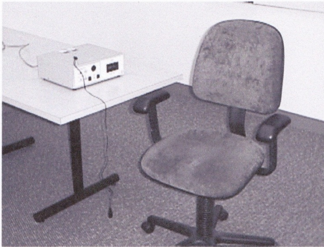
Figure 3. Test Setup to Measure Number of ESD Events
