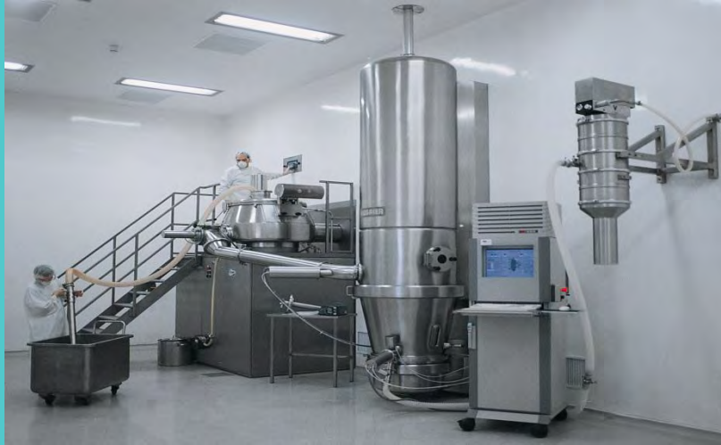
HSM discharging to FB dryer FB dryer discharge with vacuum conveying
